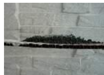
④ Results in a carbide layer of foam 40 times in size with excellent thermal insulation
