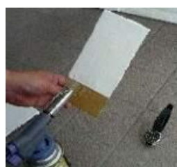
① Heating the coated surface of paint
