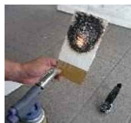
③ A carbide layer begins to form as the foaming continues
